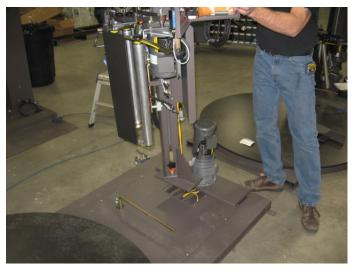
6. With the tower still suspended from the crane, thread the connection cables through the hole in the bottom of the tower.
